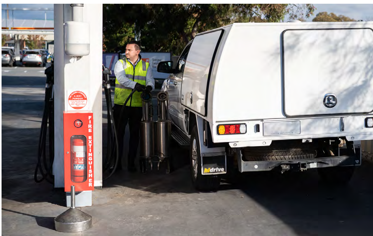
A National Measurement Institute Trade Measurement Officer tests a fuel bowser for accuracy.
